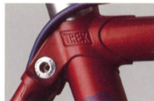
Seat stays fit into a special sleeve for a cleaner, more precise braze.
