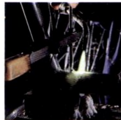
Advanced manufacturing processes and skilled hand brazing techniques join the frames at controlled low temperatures for strength and durability.
